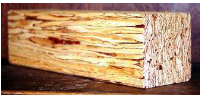
Figuur 10. Parallel Stand Lumber (Parallam)
